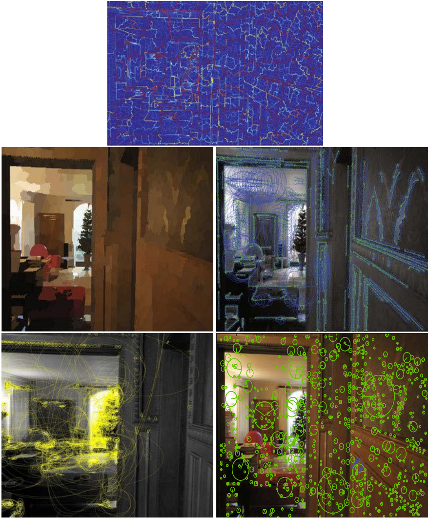
Fig. 6 Representational structures: Superpixel tree (top), dimension-two structures (color/texture regions), dimension-one structures (edges, ridges), dimension-zero structures (Harris junctions, Difference-of-Gaussian blobs). Structures are computed at all scales, and a representative subset of (multiple) scales is selected based on the local extrema of their respective detector operators (scale is color-coded in the top figure, red=coarse, blue=fine). Only a fraction of the structures detected are visualized, for clarity purposes. All structures are supported on the Representational Graph, described in the next figure.
