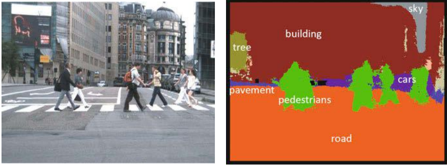
Fig. 3 Semantic segmentation. Every pixel of an input image (left) is assigned one of object categories (right).
